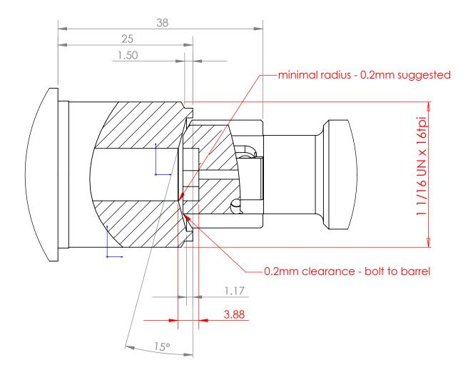
Barrel thread detail for actions from serial number \$06-001 onwards. Suggested breach for 223 case use as guidance only.
