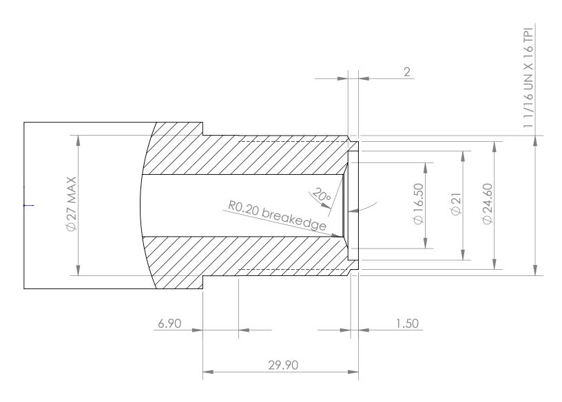
Barrel thread detail for Model 07. Suggested breach for 308 case use as guidance only.
