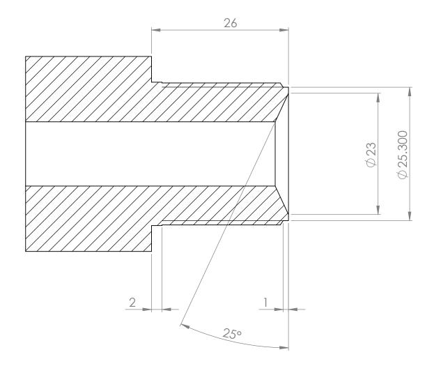
Barrel thread detail for actions from serial number P06-001 onwards. Suggested breach for 308 case use as guidance only.
