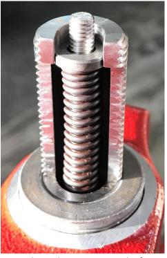
• Screw the cocking piece onto the firing pin shaft in a clockwise direction and remove the secured firing pin assembly from the loading press.
