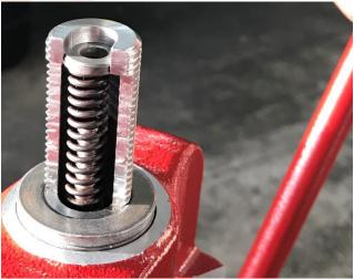
• Ensure the firing pin spring, washer hole and shaft align.
