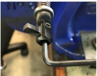
• After the cocking piece has cooled down undo anticlockwise with an adjustable wrench. Be careful while taking the cocking piece off as the spring will still have tension and will push the Firing Pin Washer and Cocking Piece off the firing pin shaft and can be lost.
