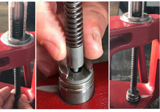
• Hold the firing pin washer onto the recess of the striker press tool while gently loading the spring up against the washer, retaining it in place.
