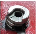
• Screw the striker press tool into the die holder of the loading press.
