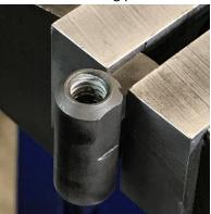
O Using an M6 x 1 tap, re-thread through the hole to clear out any Loctite still in the cocking pieced threaded hole.
