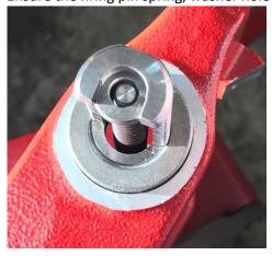
• Compress the striker spring until the threaded shaft protrudes about 10mm above the washer, be carful not to over compress the spring.
